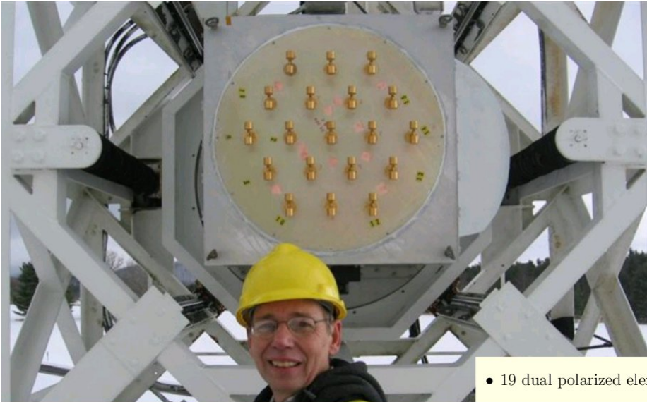
Thick, impedance-optimized dipoles, 20-meter, 2010
