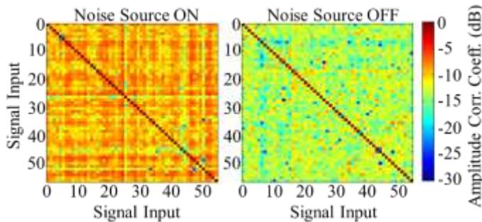
Figure 1: Absolute part of inter element correlation matrices. The noise source is turned (left) on and (right) off.
