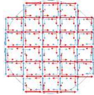
Figure 4: Dual polarized planar antenna array of 61 TSA elements.
