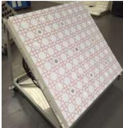
Figure: Crossed-ring antenna array working at 450MHz-1450MHz with the improved polarisation isolation and integrated LNAs
