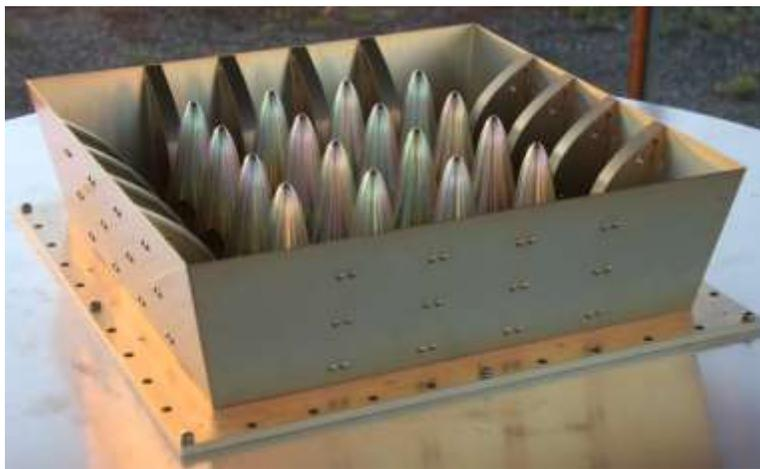
Figure 1. The 40 channel prototype array during testing at the Parkes aperture array test facility.
