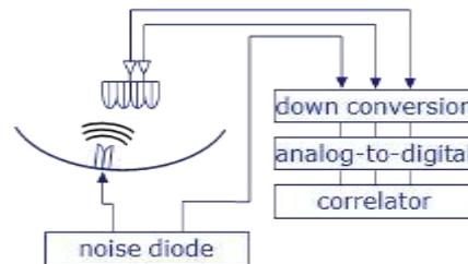
Figure 2: Block diagram of the calibration system.
