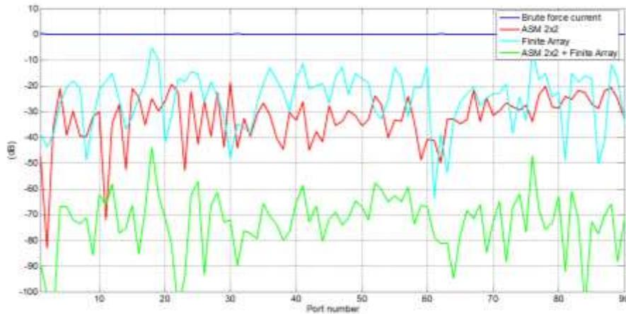
Figure 2: Comparison of the brute force port current and the error of ASM-MBF simulated currents.
