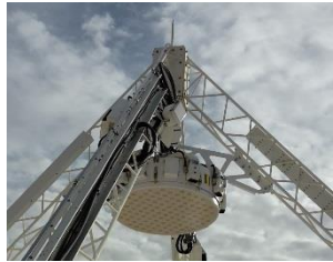
Mk-II PAF: checkerboard array, LNAs, RF filters, laser drivers
